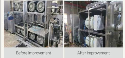
Unnecessary power consumption due to the use of a ring blower to supply air for rinse water removal in the shipment 3L secondary washer has been improved as follows:
