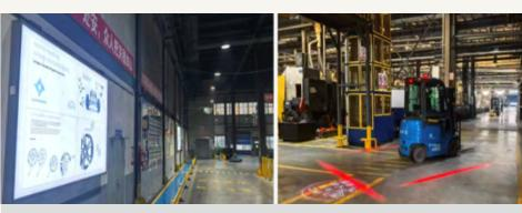
Separate pedestrian and vehicle traffic by providing distinct forklift / worker movement paths at the Longkou Hyundai Sungwoo Automotive
